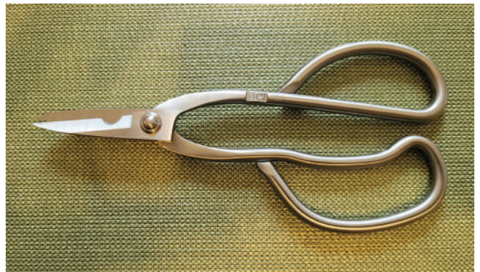
This stainless steel scissor will cut 4 mm diameter aluminum wire and branches 6 mm thick
