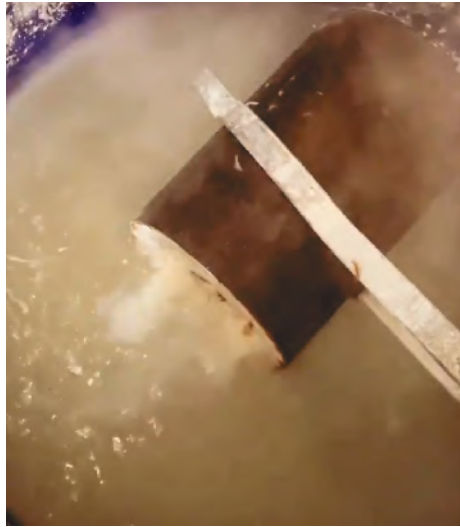
The hot flask is then placed in a tub of water to cool down.
