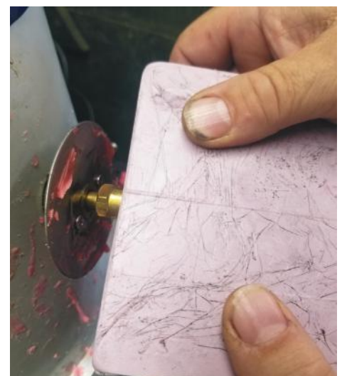
After we have a rubber mold, we can shoot hot wax under pressure into this rubber mold and duplicate our creation, as you see above.
