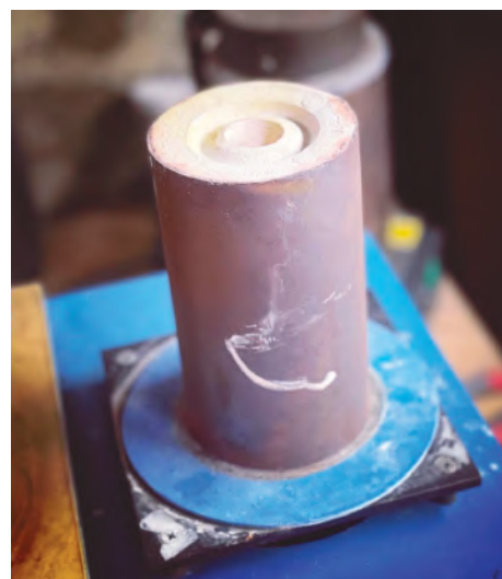
Once the molten metal is ready, the hot flask is removed from the oven and placed on the vacuum table with the hole upwards.
