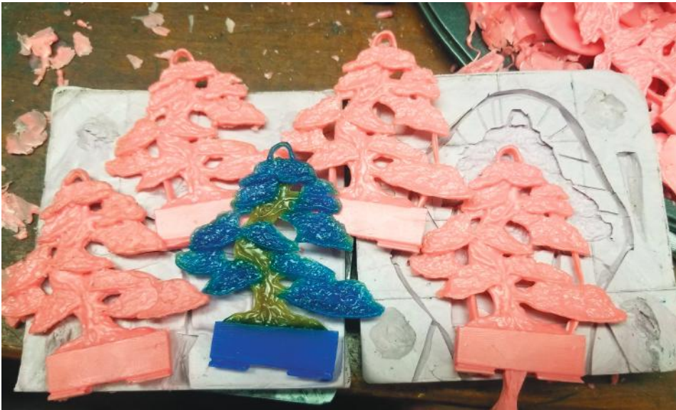
It will take about 30 minutes to clean up and detail each new wax award that comes out of our mold, and we need to ensure each is as highly detailed as the original creation.
