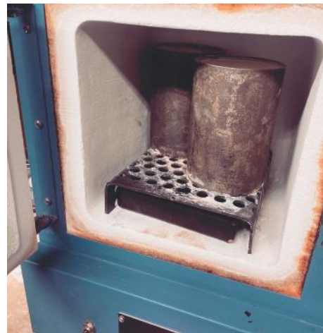
The flasks are placed in a hot oven with the wax end down. The wax is heated overnight, so all of the wax melts out.
