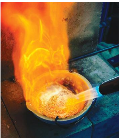
Now the bronze pellets are heated to a glowing red color.
