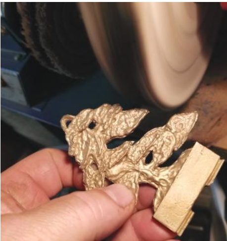
The final stage is polishing each medal with a cloth wheel.
