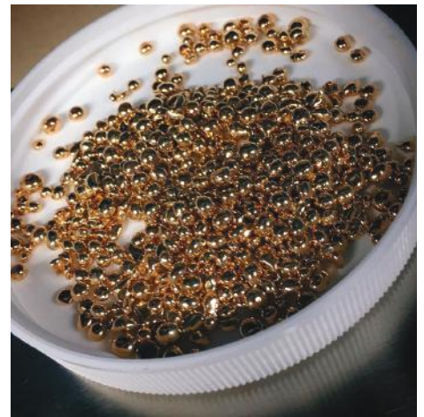
Bronze pellets are measured to the exact amount needed to fill the negative impression created by the wax melting out of the flask.
