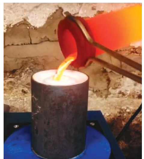
The molten metal is poured into the hot flask filling the plaster void where the wax has melted.
