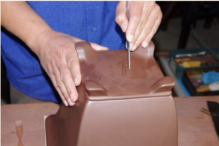
21. Locating position for drain hole.
