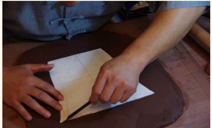
8. Using the pattern to slice the clay.
