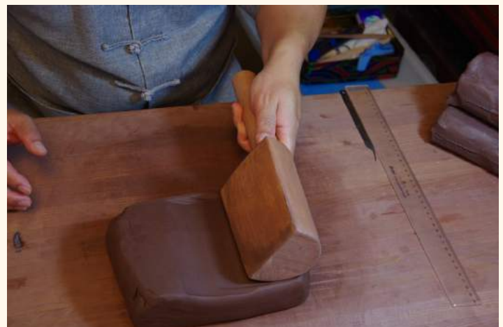
6. Hammering the clay into appropriate pieces.
