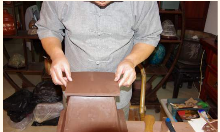
14. Joining the pot bottom to the lower part of the sides.
