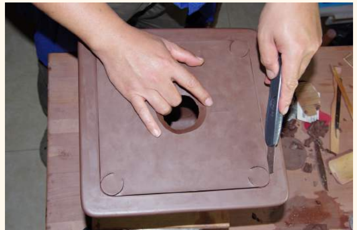
18. Cutting away the top to make the rim of the pot.
