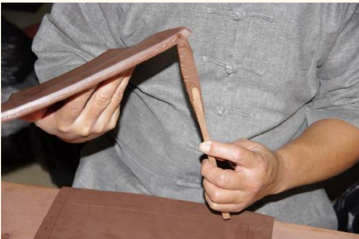
11. Applying the slurry to the edges in preparation of joining pieces.
