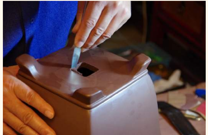
22. Cutting drain hole in bottom of pot.
