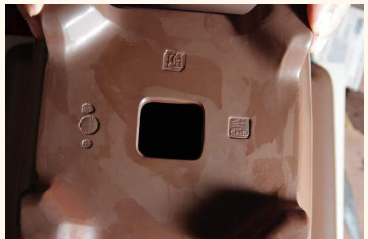
24. Finished bottom of pot with legs, drain hole, and seals.
