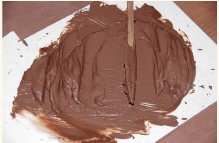
10. Getting the clay slurry to the right consistency.
