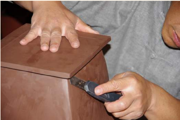
15. Trimming the newly attached bottom of the pot.
